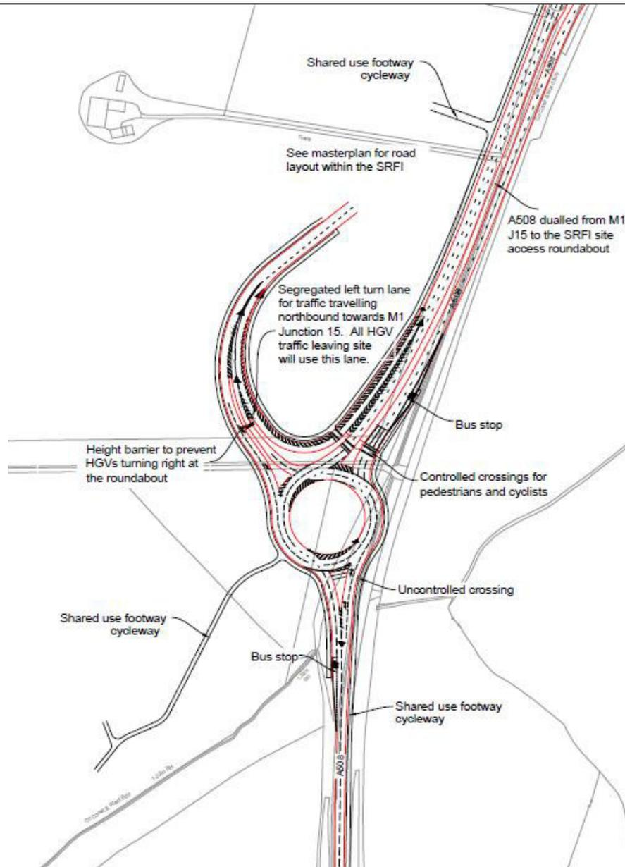
**Figure 2 – New A508 / Site Access Roundabout**
